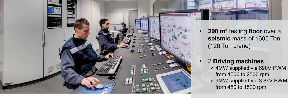
**Converter & Motor Combined Load Testing**
